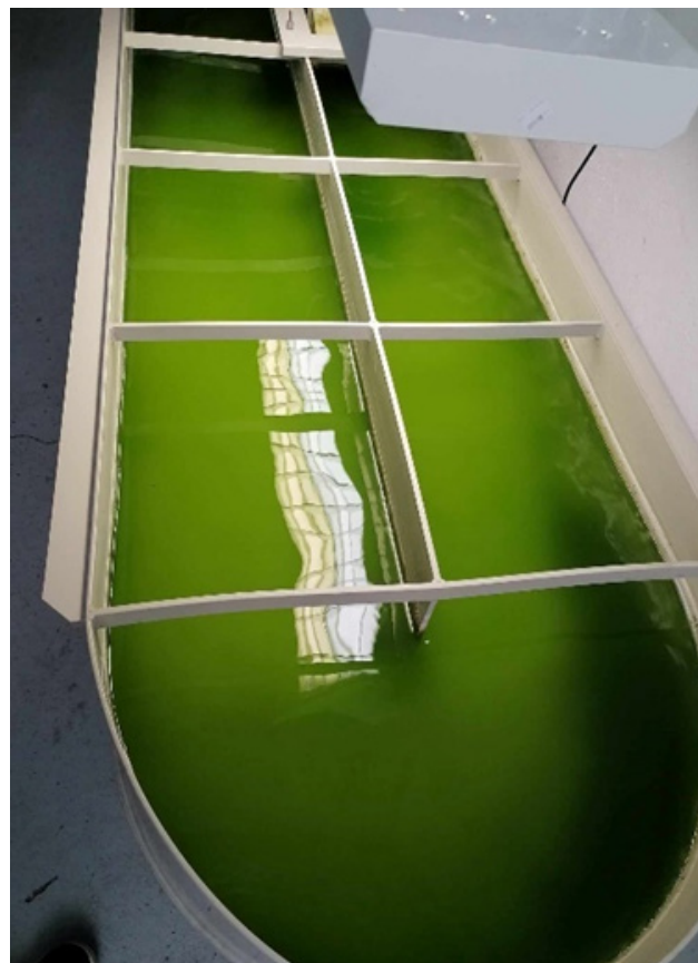
Figure 3 Photobioreactor with microalgae Chlorella sorokiniana after a week
