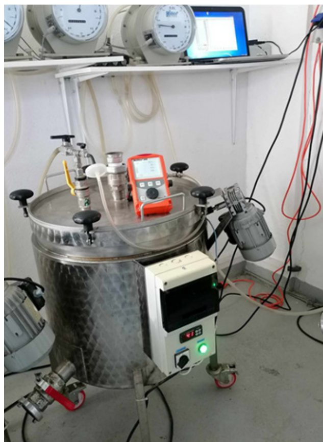
Figure 1 Fermenter 100 l with with Ritter gas meters at SAU in Nitra in year 2023
